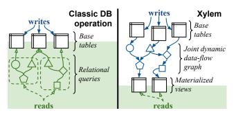
**Figure 1:** Classic databases compute read queries from base tables, while Xylem feeds writes through a dynamic, live-adapting data-flow graph to update materialize views.
